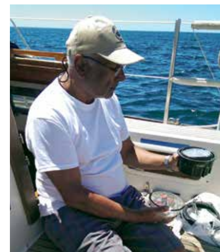
Stripping the binnacle compass down to find it had been filled with corrosive diesel fuel
