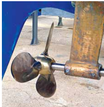
The re-worked propeller shaft and shiny new feathering propeller were fitted and ready
